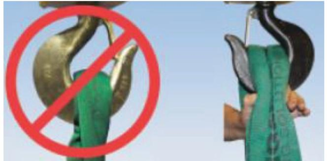
2 Squeeze both paths together to fit sling into fitting.
