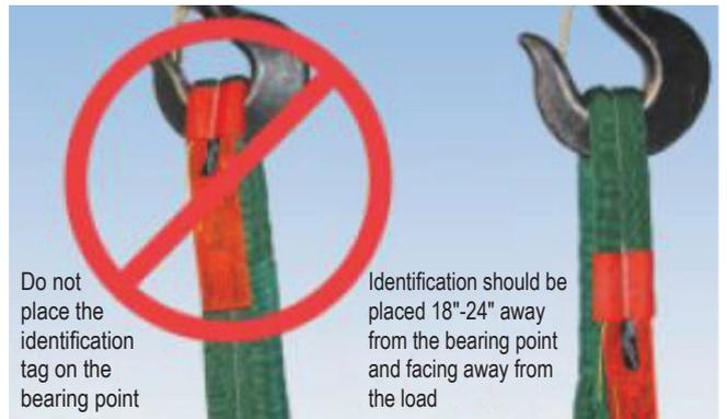
6 Place sling identification 45 - 60cm away from bearing point & facing away from load.
