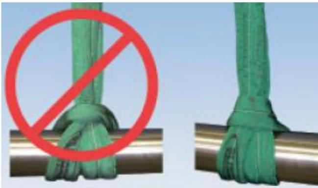
5 Sling paths should be smooth in the choker hitch without any twisting.
