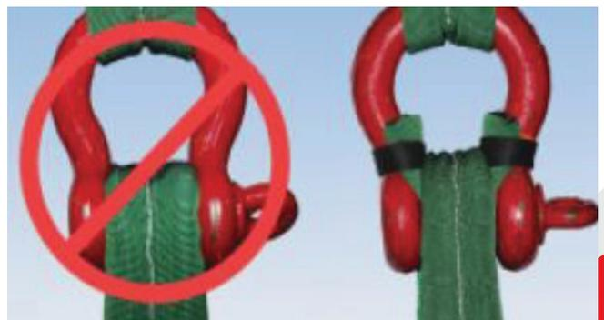
8 Use sling protection over the pin to protect the sling from cutting on the edges of the shackle's holes.
