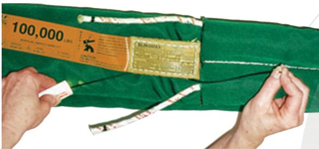
The simple fibre optic test indicates whether a sling has sustained heat or chemical damage.
